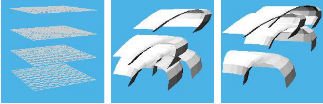
Figure 5: Arguments and corresponding graphs of a threevariate transfinite cubic Hermite map [0, 1]^3 \rightarrow E^3 which interpolates two given bivariate (surface) maps.
