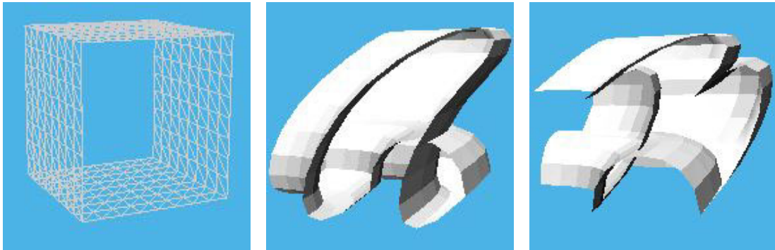
Figure 6: Arguments and corresponding graphs of a threevariate transfinite cubic Hermite map [0, 1]^3 \rightarrow E^3 which interpolates two given bivariate (surface) maps.
